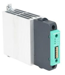
Gefran solid state relay, 35mm DIN rail mount, 6-32 VDC input voltage, SPST, (1) N.O. SCR, 40A contact rating, 24-600 VAC load voltage, push-in spring, overvoltage and thermal protection. Thermal/load interruption alarm.
