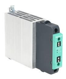
Gefran solid state relay, 35mm DIN rail mount, 20-260 VAC input voltage, SPST, (1) N.O. SCR, 40A contact rating, 24-600 VAC load voltage, push-in spring, overvoltage and thermal protection. Thermal alarm.
