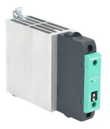
Gefran solid state relay, 35mm DIN rail mount, 20-260 VAC input voltage, SPST, (1) N.O. SCR, 40A contact rating, 24-600 VAC load voltage, push-in spring, overvoltage protection.
