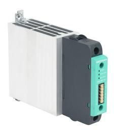
Gefran solid state relay, 35mm DIN rail mount, 6-32 VDC input voltage, SPST, (1) N.O. SCR, 40A contact rating, 24-480 VAC load voltage, push-in spring, overvoltage and thermal protection. Thermal/load interruption alarm.
