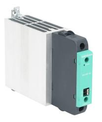
Gefran solid state relay, 35mm DIN rail mount, 6-32 VDC input voltage, SPST, (1) N.O. SCR, 40A contact rating, 24-480 VAC load voltage, push-in spring, overvoltage protection.
