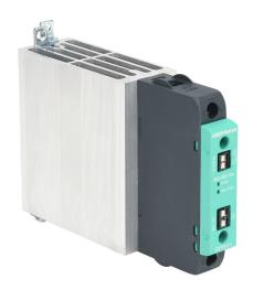
Gefran solid state relay, 35mm DIN rail mount, 20-260 VAC input voltage, SPST, (1) N.O. SCR, 40A contact rating, 24-480 VAC load voltage, push-in spring, overvoltage and thermal protection. Thermal alarm.
