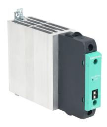
Gefran solid state relay, 35mm DIN rail mount, 20-260 VAC input voltage, SPST, (1) N.O. SCR, 40A contact rating, 24-480 VAC load voltage, push-in spring, overvoltage protection.
