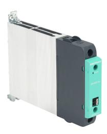
Gefran solid state relay, 35mm DIN rail mount, 6-32 VDC input voltage, SPST, (1) N.O. SCR, 30A contact rating, 24-600 VAC load voltage, push-in spring, overvoltage protection.
