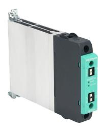
Gefran solid state relay, 35mm DIN rail mount, 20-260 VAC input voltage, SPST, (1) N.O. SCR, 30A contact rating, 24-600 VAC load voltage, push-in spring, overvoltage and thermal protection. Thermal alarm.
