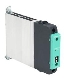
Gefran solid state relay, 35mm DIN rail mount, 20-260 VAC input voltage, SPST, (1) N.O. SCR, 30A contact rating, 24-600 VAC load voltage, push-in spring, overvoltage protection.
