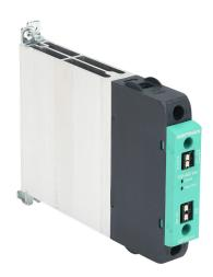
Gefran solid state relay, 35mm DIN rail mount, 20-260 VAC input voltage, SPST, (1) N.O. SCR, 30A contact rating, 24-480 VAC load voltage, push-in spring, overvoltage and thermal protection. Thermal alarm.
