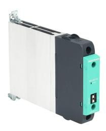
Gefran solid state relay, 35mm DIN rail mount, 20-260 VAC input voltage, SPST, (1) N.O. SCR, 30A contact rating, 24-480 VAC load voltage, push-in spring, overvoltage protection.
