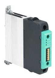
Gefran solid state relay, 35mm DIN rail mount, 6-32 VDC input voltage, SPST, (1) N.O. SCR, 25A contact rating, 24-600 VAC load voltage, push-in spring, overvoltage and thermal protection. Thermal/load interruption alarm.
