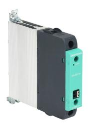
Gefran solid state relay, 35mm DIN rail mount, 6-32 VDC input voltage, SPST, (1) N.O. SCR, 25A contact rating, 24-600 VAC load voltage, push-in spring, overvoltage protection.
