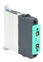
Gefran solid state relay, 35mm DIN rail mount, 20-260 VAC input voltage, SPST, (1) N.O. SCR, 25A contact rating, 24-600 VAC load voltage, push-in spring, overvoltage and thermal protection. Thermal alarm.
