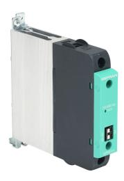
Gefran solid state relay, 35mm DIN rail mount, 20-260 VAC input voltage, SPST, (1) N.O. SCR, 25A contact rating, 24-600 VAC load voltage, push-in spring, overvoltage protection.
