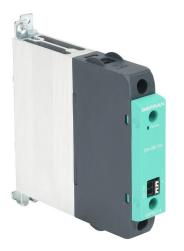
Gefran solid state relay, 35mm DIN rail mount, 6-32 VDC input voltage, SPST, (1) N.O. SCR, 25A contact rating, 24-480 VAC load voltage, push-in spring, overvoltage protection.
