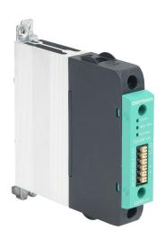
Gefran solid state relay, 35mm DIN rail mount, 6-32 VDC input voltage, SPST, (1) N.O. SCR, 15A contact rating, 24-600 VAC load voltage, push-in spring, overvoltage and thermal protection. Thermal/load interruption alarm.
