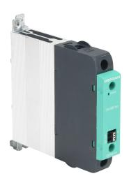
Gefran solid state relay, 35mm DIN rail mount, 6-32 VDC input voltage, SPST, (1) N.O. SCR, 15A contact rating, 24-600 VAC load voltage, push-in spring, overvoltage protection.
