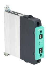
Gefran solid state relay, 35mm DIN rail mount, 20-260 VAC input voltage, SPST, (1) N.O. SCR, 15A contact rating, 24-600 VAC load voltage, push-in spring, overvoltage and thermal protection. Thermal alarm.
