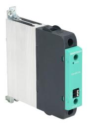
Gefran solid state relay, 35mm DIN rail mount, 6-32 VDC input voltage, SPST, (1) N.O. SCR, 15A contact rating, 24-480 VAC load voltage, push-in spring, overvoltage protection.
