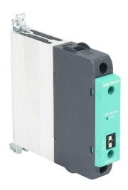
Gefran solid state relay, 35mm DIN rail mount, 20-260 VAC input voltage, SPST, (1) N.O. SCR, 15A contact rating, 24-480 VAC load voltage, push-in spring, overvoltage protection.
