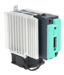
Gefran solid state relay with fan, 35mm DIN rail mount, 6-32 VDC input voltage, SPST, (1) N.O. SCR, 120A contact rating, 24-600 VAC load voltage, push-in spring, overvoltage and thermal protection. Thermal/load interruption alarm.
