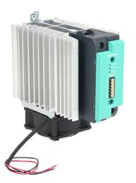
Gefran solid state relay with fan, 35mm DIN rail mount, 6-32 VDC input voltage, SPST, (1) N.O. SCR, 120A contact rating, 24-600 VAC load voltage, push-in spring, overvoltage and thermal protection, external 24 VDC required. Thermal/load interruption alarm.
