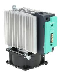
Gefran solid state relay with fan, 35mm DIN rail mount, 6-32 VDC input voltage, SPST, (1) N.O. SCR, 120A contact rating, 24-600 VAC load voltage, push-in spring, overvoltage and thermal protection, external 115 VAC required. Thermal/load interruption alarm.
