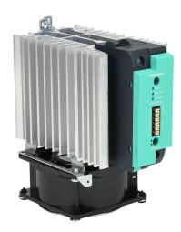
Gefran solid state relay with fan, 35mm DIN rail mount, 6-32 VDC input voltage, SPST, (1) N.O. SCR, 120A contact rating, 24-600 VAC load voltage, push-in spring, overvoltage and thermal protection, external 230 VAC required. Thermal/load interruption alarm.
