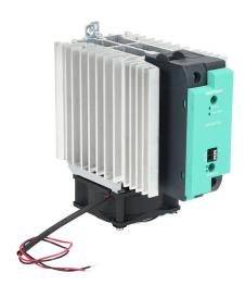
Gefran solid state relay with fan, 35mm DIN rail mount, 6-32 VDC input voltage, SPST, (1) N.O. SCR, 120A contact rating, 24-600 VAC load voltage, push-in spring, overvoltage and thermal protection, external 24 VDC required.
