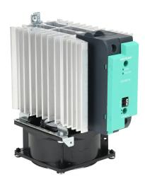
Gefran solid state relay with fan, 35mm DIN rail mount, 6-32 VDC input voltage, SPST, (1) N.O. SCR, 120A contact rating, 24-600 VAC load voltage, push-in spring, overvoltage and thermal protection, external 115 VAC required.
