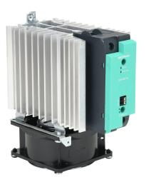
Gefran solid state relay with fan, 35mm DIN rail mount, 6-32 VDC input voltage, SPST, (1) N.O. SCR, 120A contact rating, 24-600 VAC load voltage, push-in spring, overvoltage and thermal protection, external 230 VAC required.
