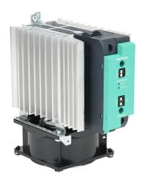
Gefran solid state relay with fan, 35mm DIN rail mount, 20-260 VAC input voltage, SPST, (1) N.O. SCR, 120A contact rating, 24-600 VAC load voltage, push-in spring, overvoltage and thermal protection, external 115 VAC required. Thermal alarm.
