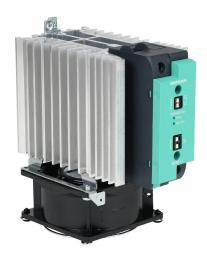
Gefran solid state relay with fan, 35mm DIN rail mount, 20-260 VAC input voltage, SPST, (1) N.O. SCR, 120A contact rating, 24-600 VAC load voltage, push-in spring, overvoltage and thermal protection, external 230 VAC required. Thermal alarm.
