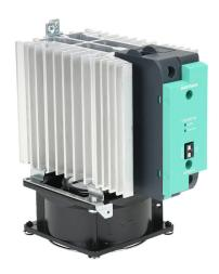
Gefran solid state relay with fan, 35mm DIN rail mount, 20-260 VAC input voltage, SPST, (1) N.O. SCR, 120A contact rating, 24-600 VAC load voltage, push-in spring, overvoltage and thermal protection, external 115 VAC required.
