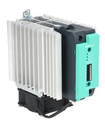
Gefran solid state relay with fan, 35mm DIN rail mount, 6-32 VDC input voltage, SPST, (1) N.O. SCR, 120A contact rating, 24-480 VAC load voltage, push-in spring, overvoltage and thermal protection. Thermal/load interruption alarm.
