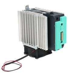
Gefran solid state relay with fan, 35mm DIN rail mount, 6-32 VDC input voltage, SPST, (1) N.O. SCR, 120A contact rating, 24-480 VAC load voltage, push-in spring, overvoltage and thermal protection, external 24 VDC required. Thermal/load interruption alarm.
