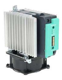
Gefran solid state relay with fan, 35mm DIN rail mount, 6-32 VDC input voltage, SPST, (1) N.O. SCR, 120A contact rating, 24-480 VAC load voltage, push-in spring, overvoltage and thermal protection, external 115 VAC required. Thermal/load interruption alarm.
