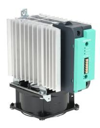
Gefran solid state relay with fan, 35mm DIN rail mount, 6-32 VDC input voltage, SPST, (1) N.O. SCR, 120A contact rating, 24-480 VAC load voltage, push-in spring, overvoltage and thermal protection, external 230 VAC required. Thermal/load interruption alarm.
