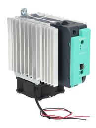
Gefran solid state relay with fan, 35mm DIN rail mount, 6-32 VDC input voltage, SPST, (1) N.O. SCR, 120A contact rating, 24-480 VAC load voltage, push-in spring, overvoltage and thermal protection, external 24 VDC required.
