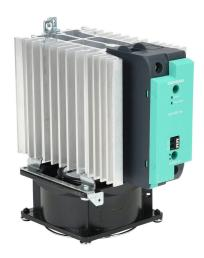
Gefran solid state relay with fan, 35mm DIN rail mount, 6-32 VDC input voltage, SPST, (1) N.O. SCR, 120A contact rating, 24-480 VAC load voltage, push-in spring, overvoltage and thermal protection, external 115 VAC required.
