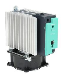
Gefran solid state relay with fan, 35mm DIN rail mount, 6-32 VDC input voltage, SPST, (1) N.O. SCR, 120A contact rating, 24-480 VAC load voltage, push-in spring, overvoltage and thermal protection, external 230 VAC required.
