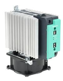
Gefran solid state relay with fan, 35mm DIN rail mount, 20-260 VAC input voltage, SPST, (1) N.O. SCR, 120A contact rating, 24-480 VAC load voltage, push-in spring, overvoltage and thermal protection, external 115 VAC required. Thermal alarm.
