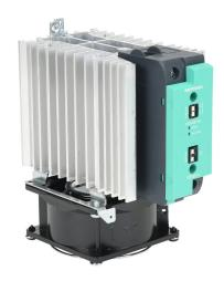
Gefran solid state relay with fan, 35mm DIN rail mount, 20-260 VAC input voltage, SPST, (1) N.O. SCR, 120A contact rating, 24-480 VAC load voltage, push-in spring, overvoltage and thermal protection, external 230 VAC required. Thermal alarm.
