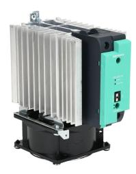
Gefran solid state relay with fan, 35mm DIN rail mount, 20-260 VAC input voltage, SPST, (1) N.O. SCR, 120A contact rating, 24-480 VAC load voltage, push-in spring, overvoltage and thermal protection, external 115 VAC required.
