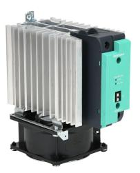
Gefran solid state relay with fan, 35mm DIN rail mount, 20-260 VAC input voltage, SPST, (1) N.O. SCR, 120A contact rating, 24-480 VAC load voltage, push-in spring, overvoltage and thermal protection, external 230 VAC required.
