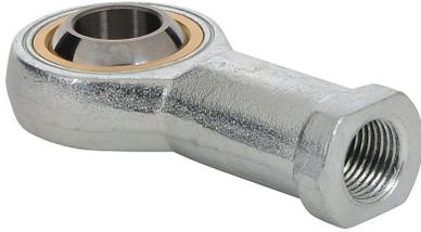
NITRA rod eye, M16 X 1.5 thread, spherical bearing, zinc plated steel. For use with G-series cylinders.
