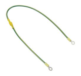
Hammond enclosure grounding strap, 22in length, 10 AWG, (2) #10-1/4in ring terminals. Package of 1. Quick-disconnect terminals, #10-32 and 1/4-20 screws, washers and nuts included.
