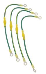
Hammond enclosure grounding strap, 12in length, 10 AWG, (2) #10-1/4in ring terminals. Package of 4. Quick-disconnect terminals, #10-32 and 1/4-20 screws, washers and nuts included.
