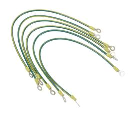
Hammond enclosure grounding strap, 16in length, 10 AWG, (2) #10-1/4in ring terminals. Package of 6. #10-32 and 1/4-20 screws, washers and nuts included.
