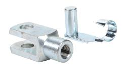
NITRA rod clevis, M20 X 1.5 thread, zinc plated steel. For use with G-series cylinders.
