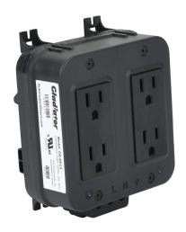
Gladiator quad straight blade receptacle, 15A, 125 VAC, 1-phase, 2-pole, 3-wire, glass fiber reinforced polyamide housing, panel or 35mm DIN rail mount.
