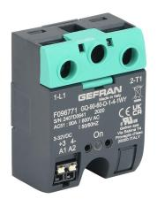
Gefran solid state relay, panel mount, 3-32 VDC input voltage, SPST, (1) N.O. SCR, 90A contact rating, 48-600 VAC load voltage, push-in spring, overvoltage protection. Thermal mounting pad included.
